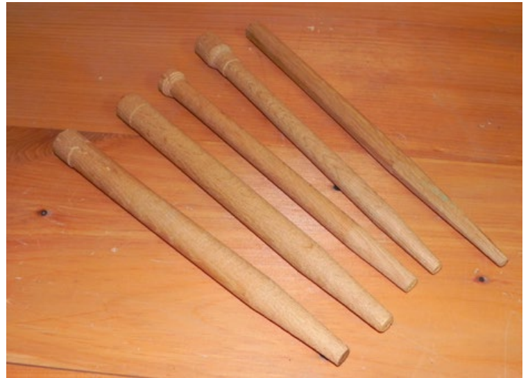
10 Manufactured pegs. On the left, 1-in. and \frac{3}{4} -in. turned pegs. On the right, a sawn octagonal one. All have a long, gradually tapered point, essential for drawboring. Some cross-grain runout is visible on each of the turned pegs.
