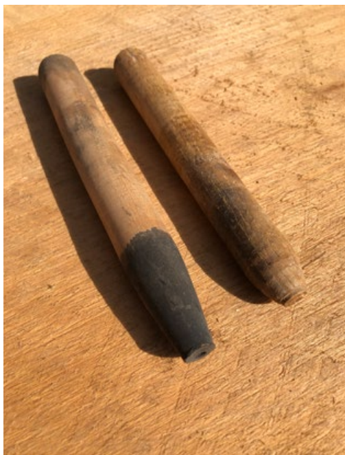
9 Old turned pegs. On the left is a 1x8-in. sugar maple peg with a gradual point (blackened from soot). On the right, a 1x7-in. blunt-pointed white ash peg. Neither has any measurable taper along its length.
