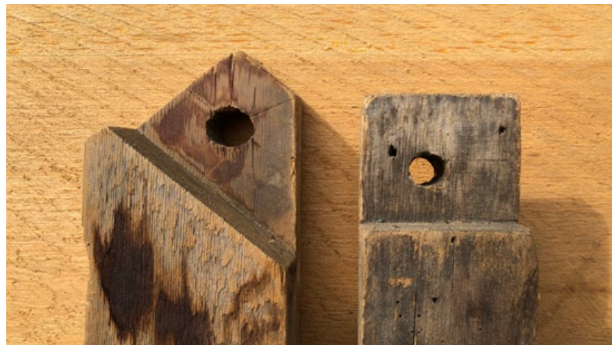
5 On the left is a 3x4 red spruce ( Picea rubens ) brace end, cut about 1855, its 3-in.-long tenon showing a 1-in. peg hole, 1\frac{1}{2} in. off the shoulder and 1\frac{1}{2} in. from the bearing nose. The hole is offset diagonally along the axis of the brace about \frac{1}{8} in.
