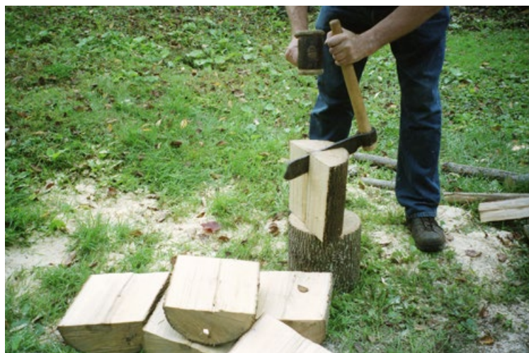
6 Riving white ash billets with a froe.
