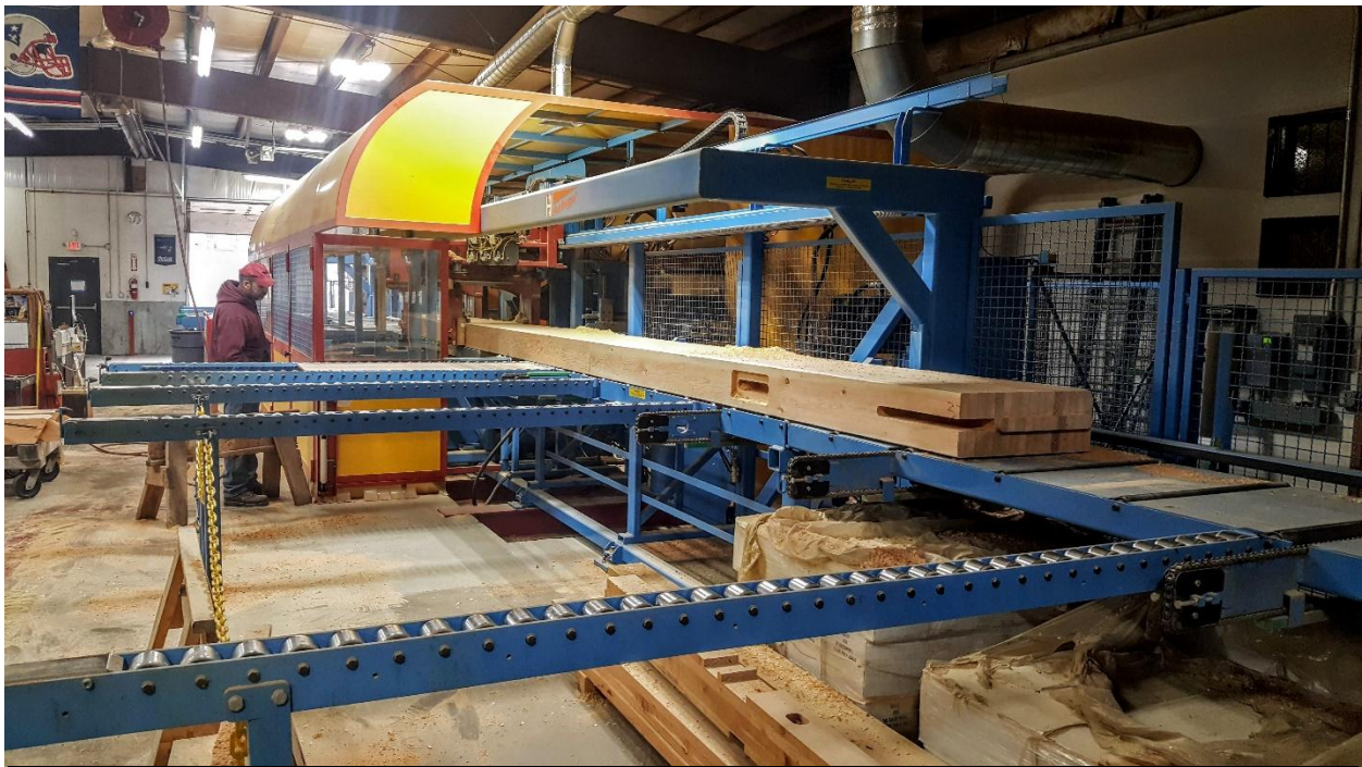
The Hundegger CNC fabricator in action Photo credit – South County Post & Beam
