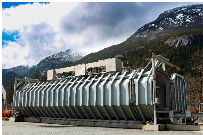
Radio frequency kiln Photo credit – FraserWood Industries
