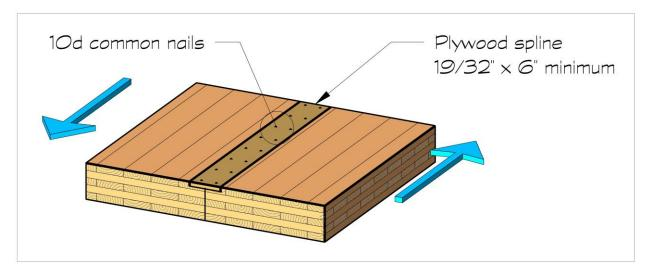
There has been some dynamic testing performed of spline joints with screw fasteners at the University of British Columbia. The research suggests that spline joints with inclined screws loaded axially typically exhibit high initial stiffness and ultimate static capacity, but are prone to non-ductile failure. Spline joints with screws installed at 90 degrees and loaded in shear, exhibited lower initial stiffness and ultimate static capacity but failed in a more ductile fashion.
