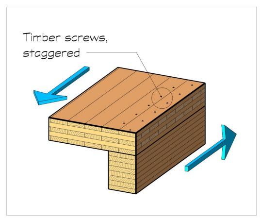
The allowable shear capacity of timber screws fastening CLT panels to timber beams is shown in Table 3. The values in the table are based on timber screws with a minimum  $F_{yb}$  of 136.6 ksi, a CLT specific gravity of 0.42 and a timber beam specific gravity of 0.49. The load is assumed to be applied parallel to the grain of the timber beam. These values have been increased for a load duration factor,  $C_D$  of 1.6 and a diaphragm adjustment factor,  $C_{di}$  of 1.1
