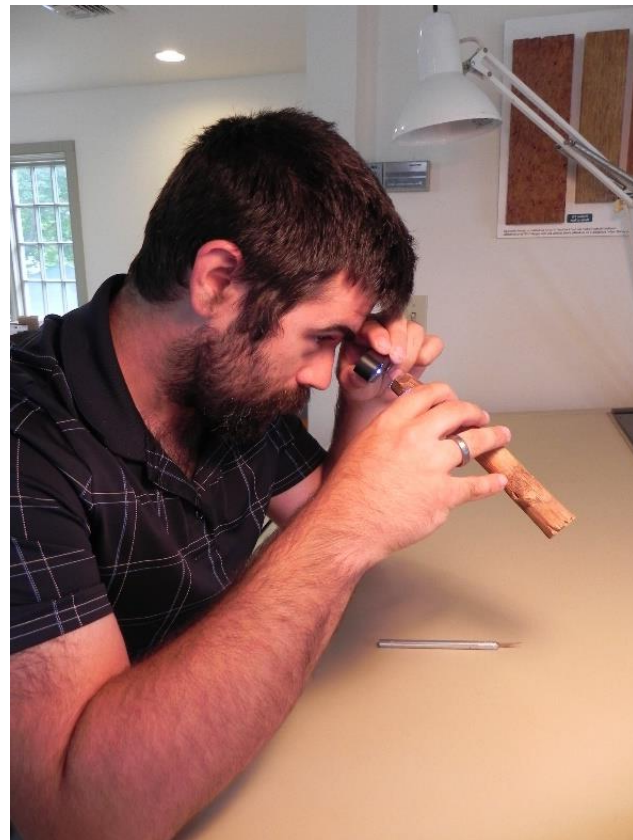
Figure 22 A hand lens is used to examine the anatomical features of a wood specimen
