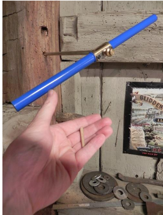
Figure 20 A specimen extracted from a timber with an increment borer
