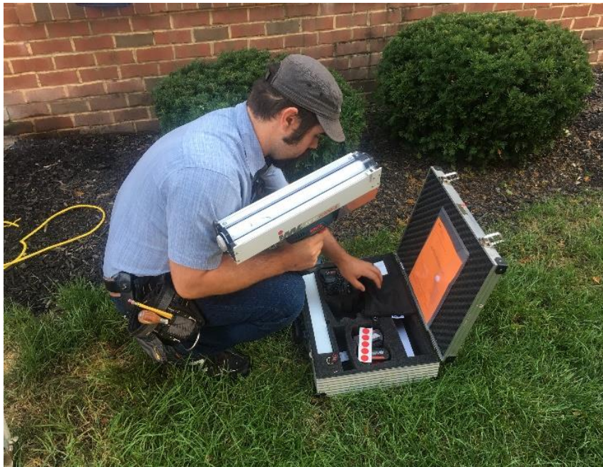
Figure 15 A resistance drill is a useful tool for identifying deterioration hidden below the surface
