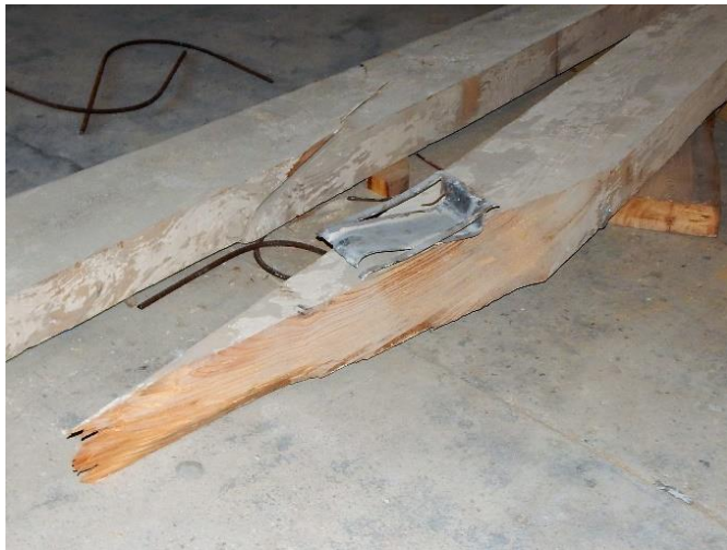
Figure 27 Failure due to excessive slope of grain
