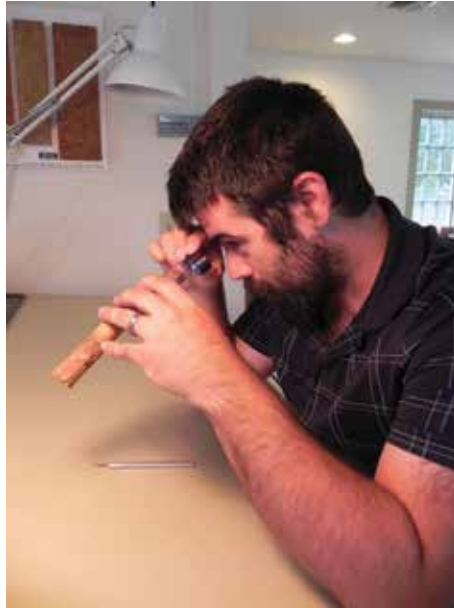
Examining the end grain of a timber specimen with a hand lens to identify the wood species.
