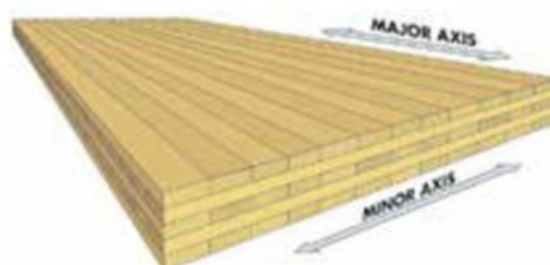
CLT panels are available up to 10 feet wide and over 60 feet long. Courtesy of WoodWorks.
