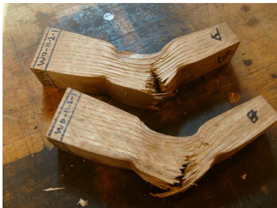
Figure 6 Crushing and Bending of Key Wedges
